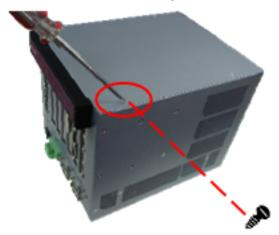
Step 4 Open the top cover and locate the two Hard Disk Drives from the side.
